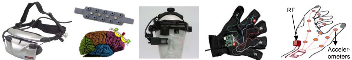
Fig.9 (1) HDT [xx] (2) fNIR band [xx] (3) Eye Tracker [xx] (4) Digital Glove [xx] (5) Glove study model
