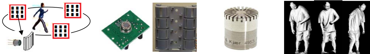
Fig.16 (1) Gait sensor array; (2) Pyroelectric sensor & lens; (3) Acoustic sensor; (4) Disorder / imbalance
