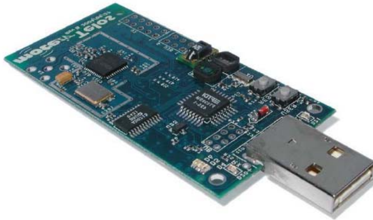
Figure 2.9 Telos (a type of mote) with IEEE 802.15.4 wireless transceiver. [Joseph05]
