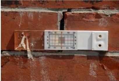
Mechanical strain gauge used to measure the growth of a crack in a masonry foundation. This one is installed on the Hudson-Athens Lighthouse. Photo by Roy Smith, used with permission.
