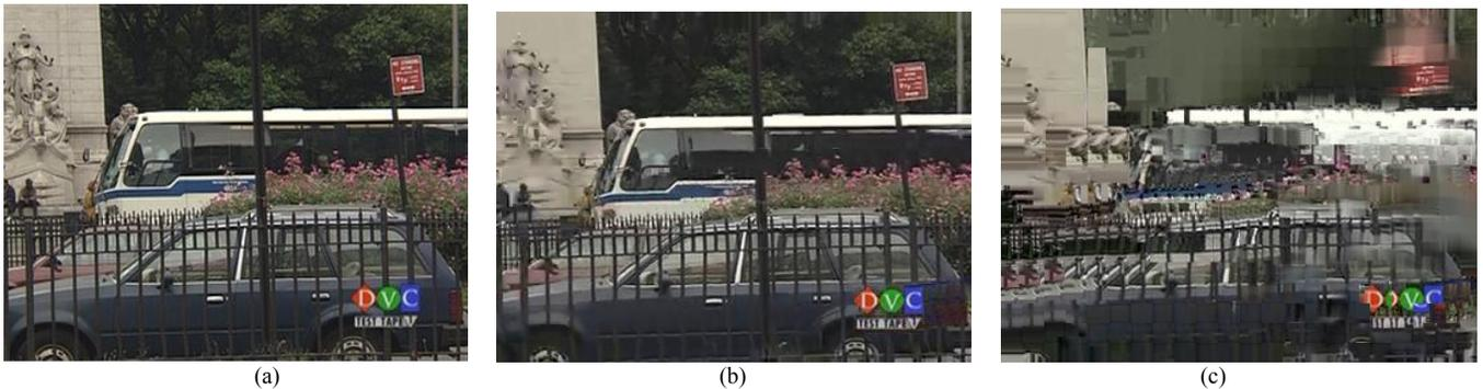
Fig.17 The quality of reconstructed video frame: (a) original video frame No.18; (b) reconstructed frame using our proposed algorithm; (c) reconstructed frame using the equal-packet loading algorithm without spectrum sensing during packet transmission.
