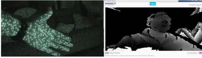
Fig. 11. (Left) IR pattern from the IR emitter of the Kinect. (Right) Depth map generated by Kinect.
