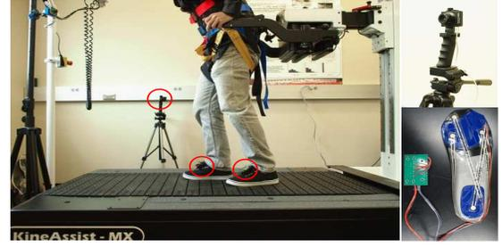
Fig. 7. The experiment setup (with the KineAssist robot treadmill) and the sensors.
