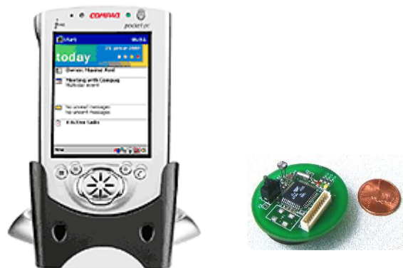
Figure 2. (left) iPAQ (right) Mica2Dot sensors
